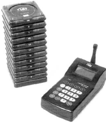
FIGURE 7-14 Coaster Pager: A coaster pager alerts the guest that his or her table is ready. Courtesy of Long Range Systems, Inc.
